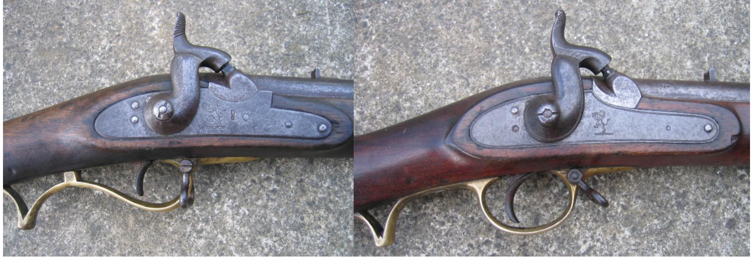
c1833? BEIC flintlock musket converted to percussion from c1837?
