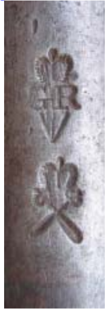
George III crown engraved on lock plate Proof marks stamped on barrel Later type George III crown proof marks stamped on barrel
