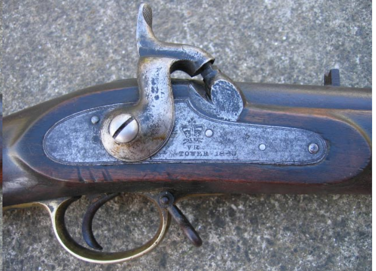
Pattern 1842 new design percussion musket fitted with P1853 hammer
