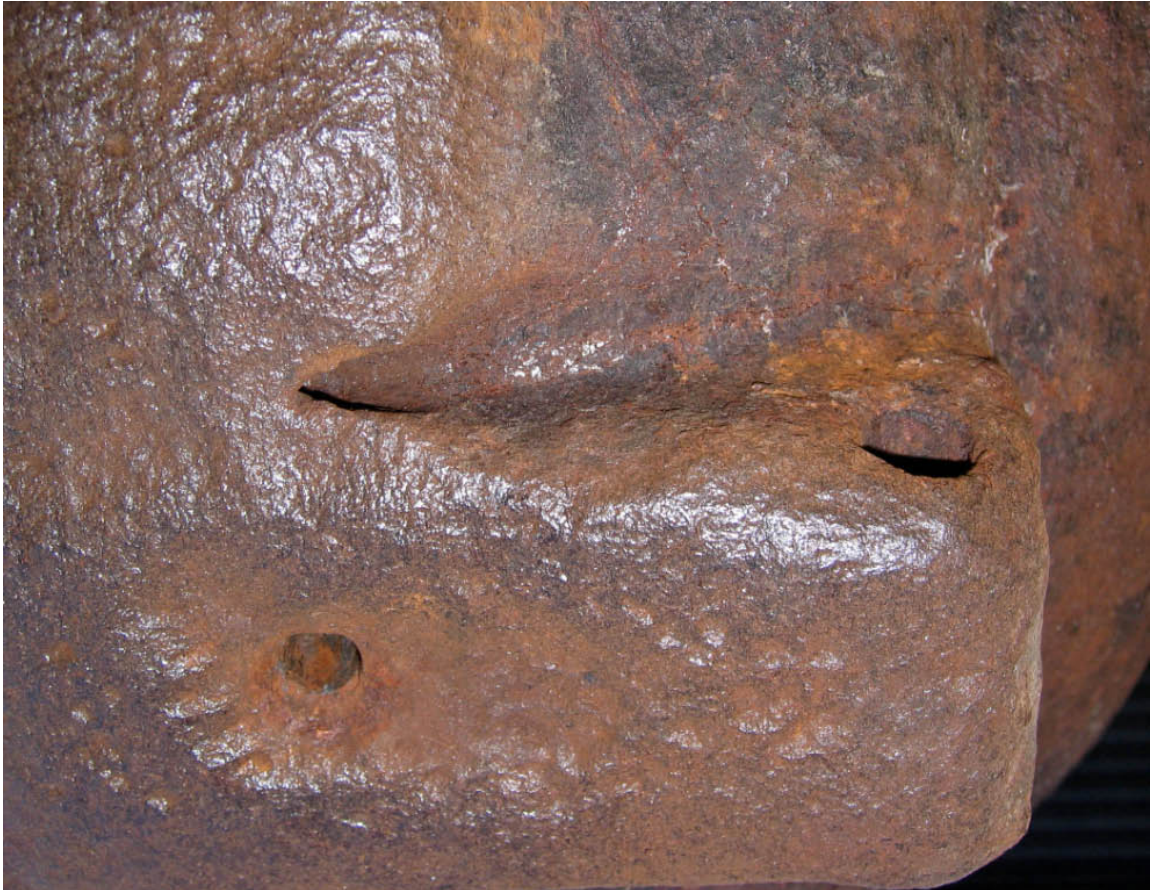
After water blasting and wire brushing (shiny areas) and vent hole drilled out. Flintlock igniter forward location (vee hole at top) and rear locking pin hole at rear of vent lump clearly visible.
