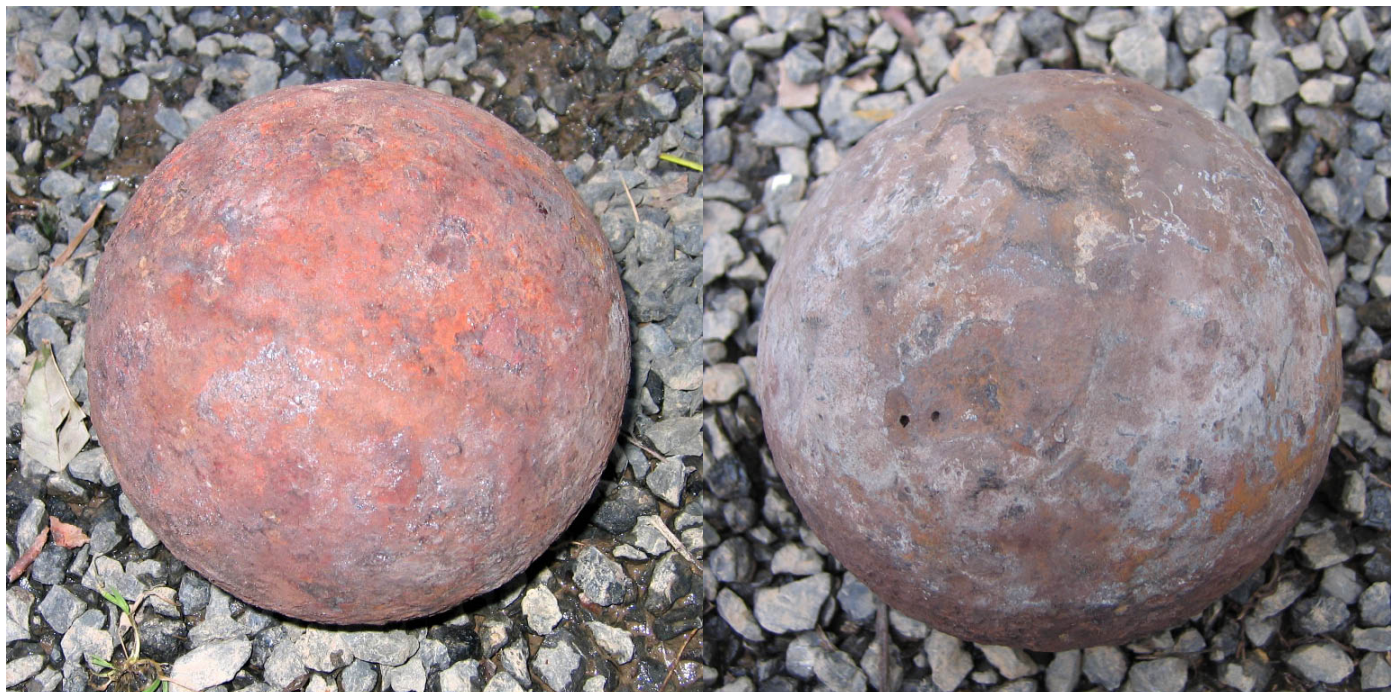
Left image: Ball as removed (still hot) showing side facing powder chamber. Compared to right image: outer side (rust flaked off) with bore / chamfer contact join line (lower) and showing small casting imperfections (holes). The standard nominal ball diameter c1800 for an 18 pounder was 5.04". This ball measured 5.08" maximum diameter includes light surface rust.
